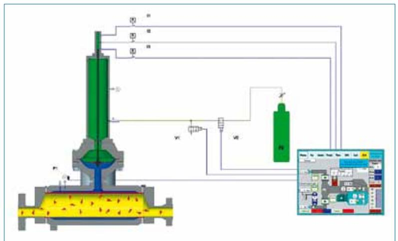
Fig. 6: Hose-diaphragm pulsation dampener with automatic adaptation to the working pressure
