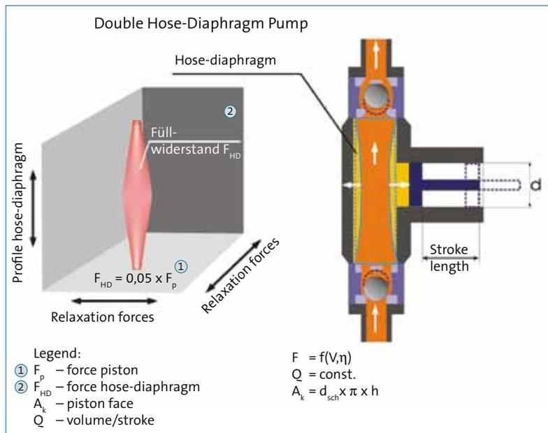
Fig. 2.2: Filling behaviour of double hose-diaphragm pumps
