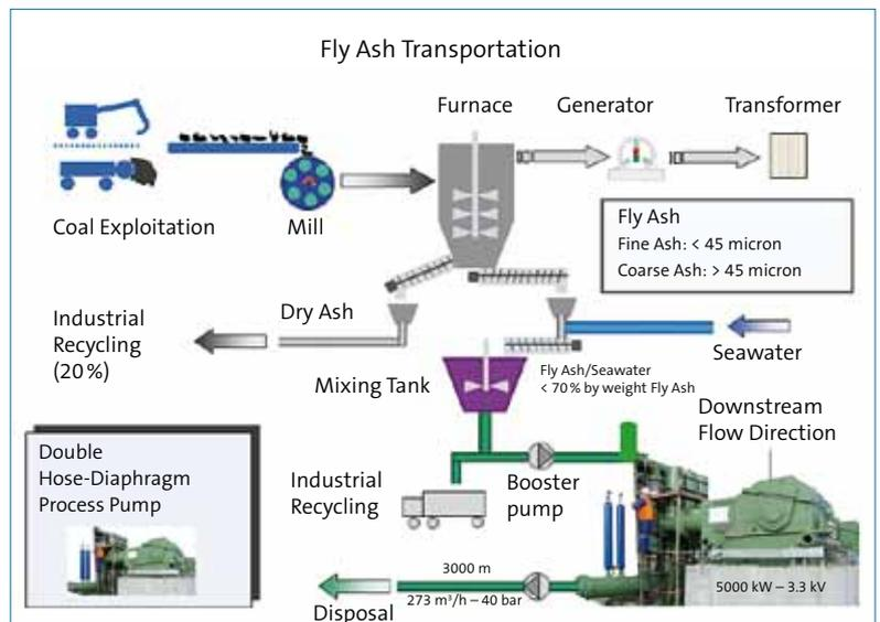
Fig. 1: Hydraulic transport system for the disposal of fly ash from coal-fired power plants
