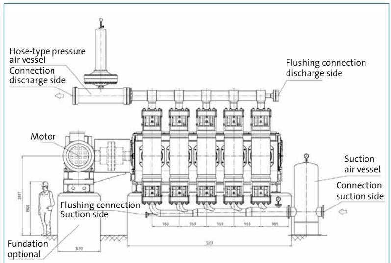
Fig. 5 : Double hose-diaphragm pumps in quintuplex design · flowrate 525 m³/h at 38 strokes/min. · driving power 2,200 kW
