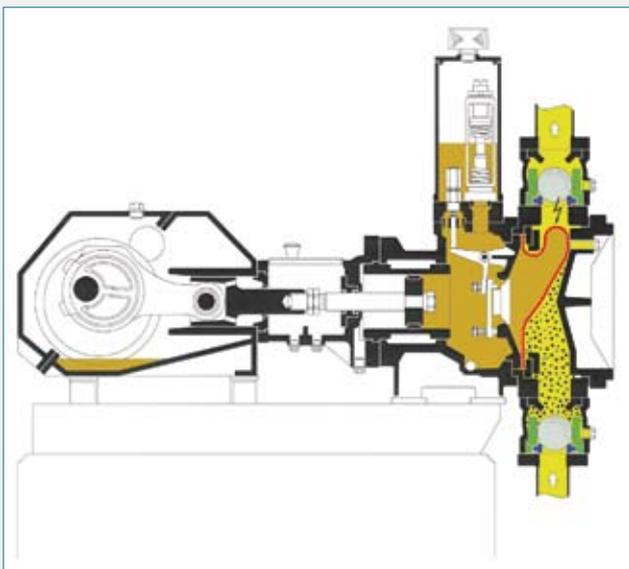
Fig. 3: Diaphragm failure as a result of sedimentation
