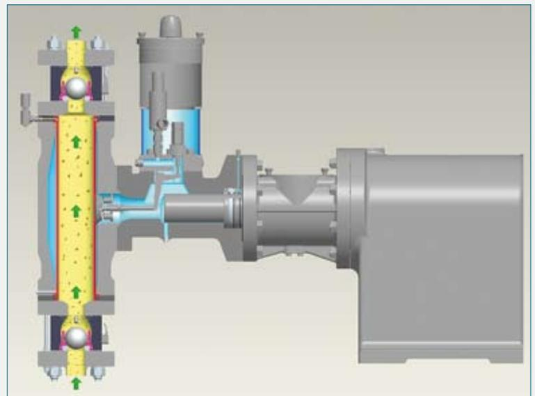
Fig. 4: Double hose-diaphragm pump
