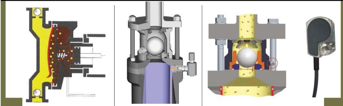
the slurry. The slurry is directed in and out of the pump via large abrasive-resistant coated steel ball-type slurry check valves.
