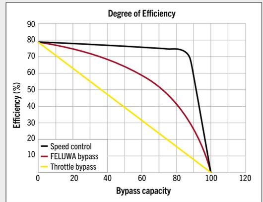
Fig. 5: Efficiency curves for different flow control systems.
