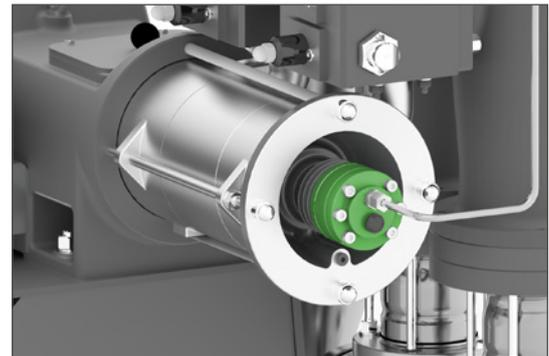
Fig. 9: The extended piston rod can serve as piston compressor to ensure continuous filling of the air vessel.
