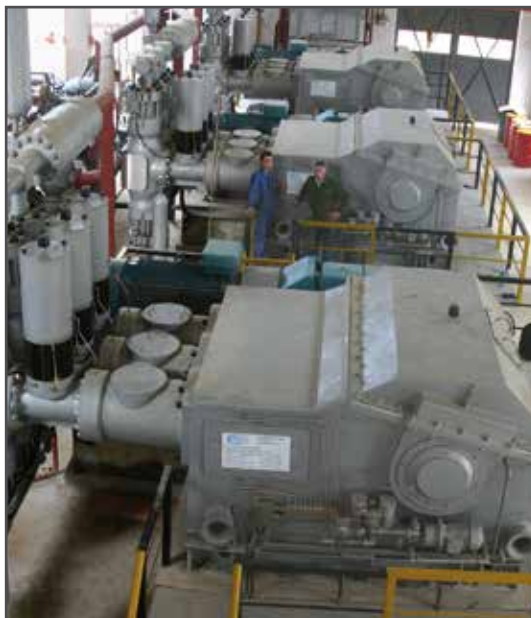
Each of the six FELUWA MULTISAFE® pumps transfers red mud at 95 m 3 /hr and 120 bar pressure at an alumina refinery in China.
